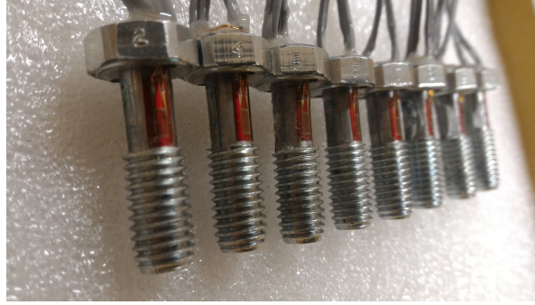
Figure 5: Bolts instrumented with strain gauge.
