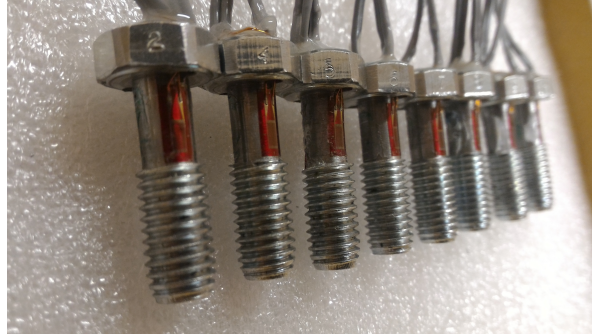
Figure 5: Bolts instrumented with strain gauge.
