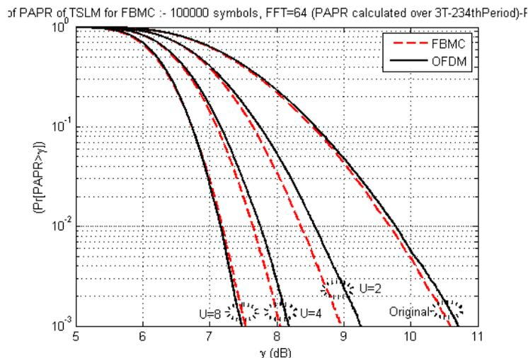
Figure 5-9: CCDF of PAPR plot for  $10^5$  FBMC symbols with PAPR calculated over  $[T, 4T]$  with  $U = 2, 4, 8$  to illustrate the impact of size of  $U$  on the TSLM scheme in comparison with SLM scheme for OFDM.
