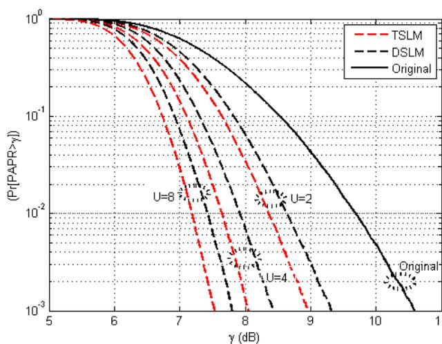
Figure 5-10: CCDF of PAPR plot for  $10^5$  FBMC symbols with PAPR calculated over  $[T, 4T]$  with  $U = 2, 4, 8$  to illustrate the comparison of the TSLM scheme with the earlier proposed DSLM scheme.
