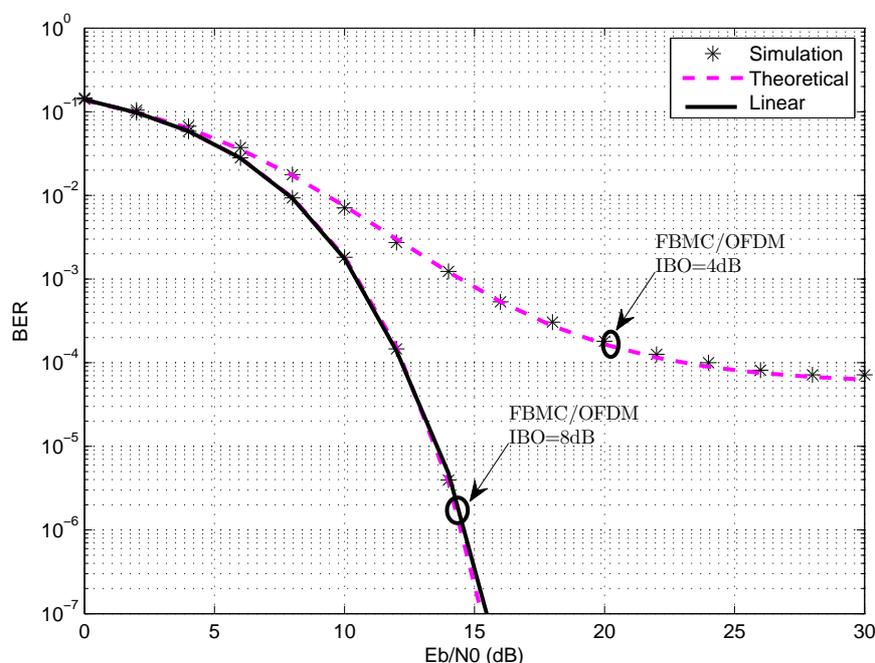
Figure 3-3: BER vs  $Eb/N_0$  for OFDM and FBMC system. SEL,  $A_{sat} = 1$ , 64 subcarriers, 16QAM, and AWGN channel.
