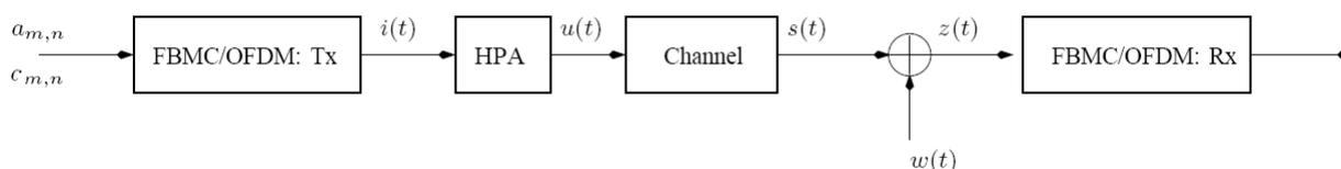
Figure 2-1: The transmission system model with NL HPA.
