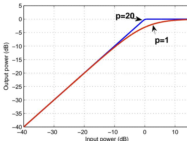
Figure 2-3: AM/AM characteristics of Rapp HPA model.
