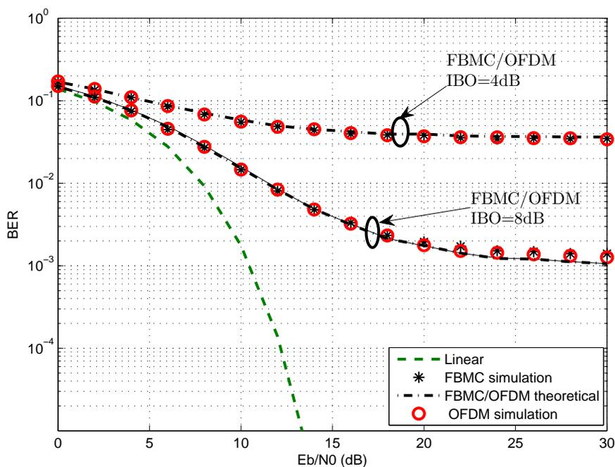
Figure 3-4: BER vs  $E_b/N_0$  for OFDM and FBMC system. Saleh HPA model, 64 subcarriers, 16QAM,  $\varphi_0 = 0$ , and AWGN channel.
