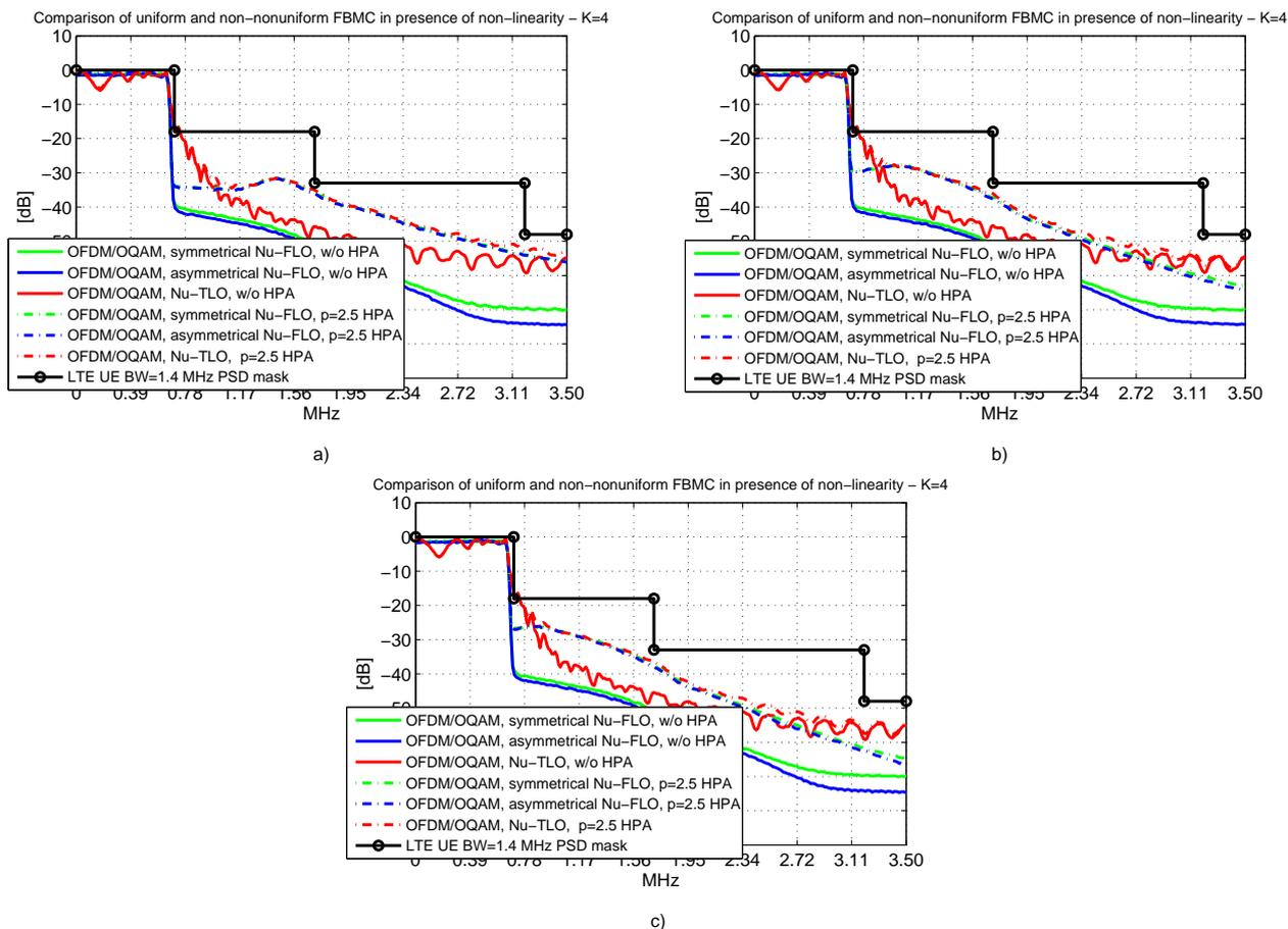
Figure 6-20: Comparison of non-uniform FLO FBMC, TLO FBMC and CP-OFDM in context of HPA and mask fitting with transmit signal spectrum cutoff; a) 1/2 spectrum cutoff, b) 1/4 spectrum cutoff c) 1/8 spectrum cutoff.
