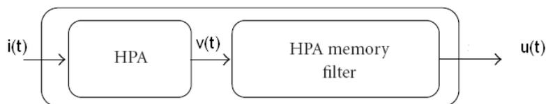
Figure 2-5: Hammerstein model for a HPA with memory.
