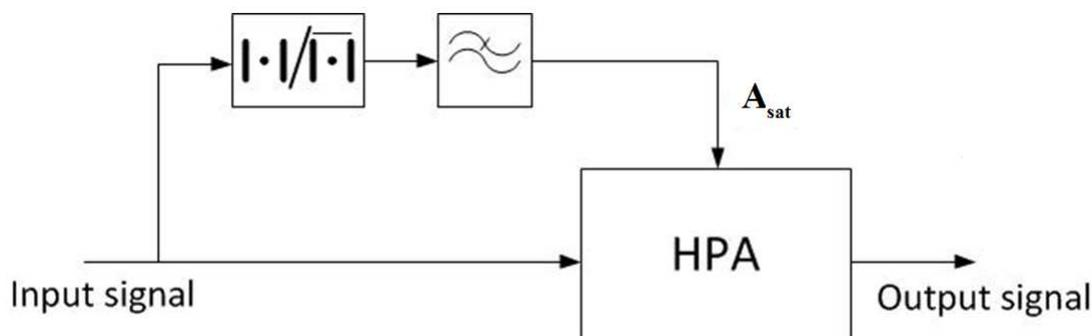
Figure 6-17: The NL HPA model controlled by filtered normalized signal envelope.
