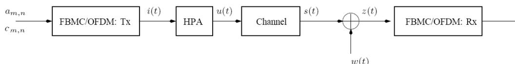
Figure 3-1: The transmission system model with FBMC and OFDM modulations.
