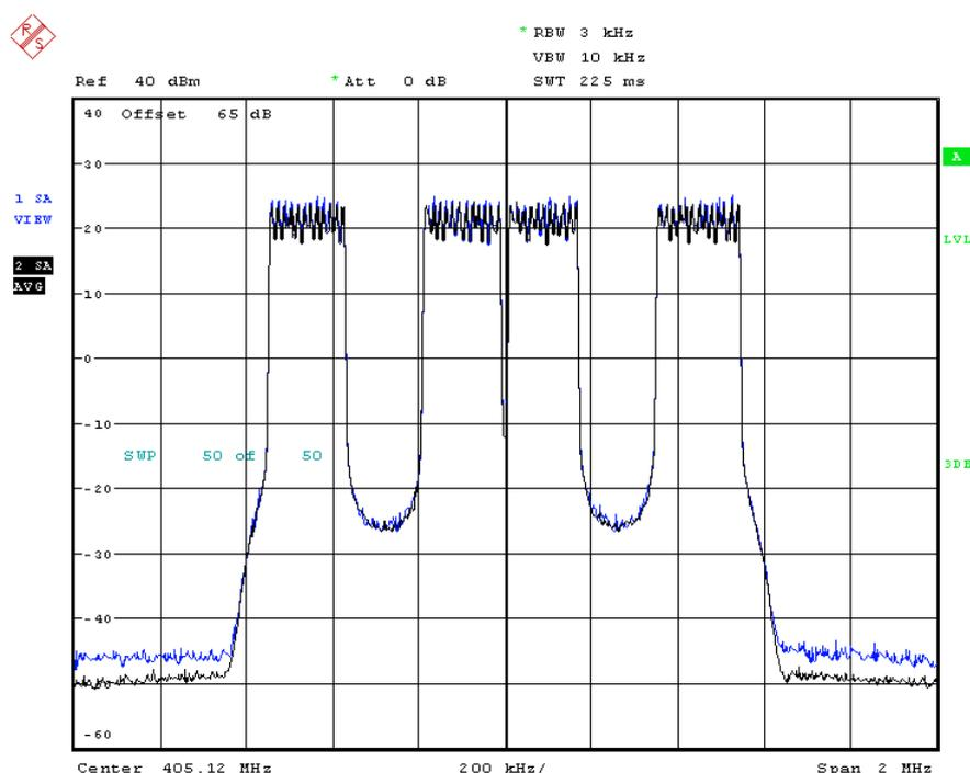
Figure 6-22: First waveform measured PSDs. At HPA base station output in blue and at *R&S SMU200* output in black.
