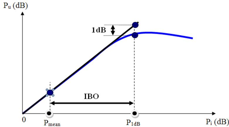
Figure 2-2: Linearized HPA and input signal with low PAPR.
