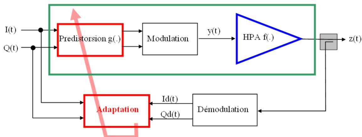
Figure 6-3: Architecture of a predistortion working in baseband.
