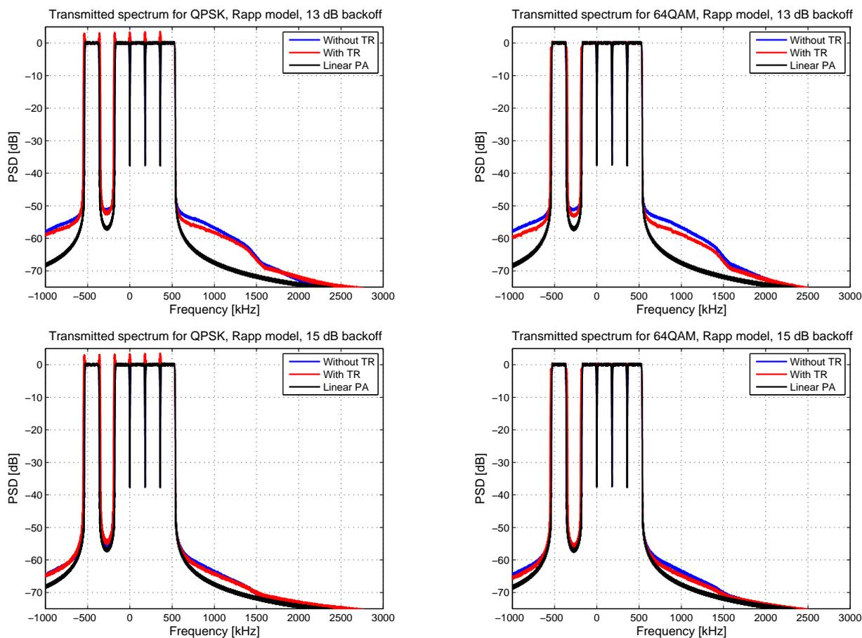
Figure 6-14: Spectral regrowth with 1.4 MHz LTE-like FBMC waveform with QPSK and 64QAM modulations and different back-off values using Rapp HPA model ( $p=2.25$ ) with or without TR based PAPR mitigation.
