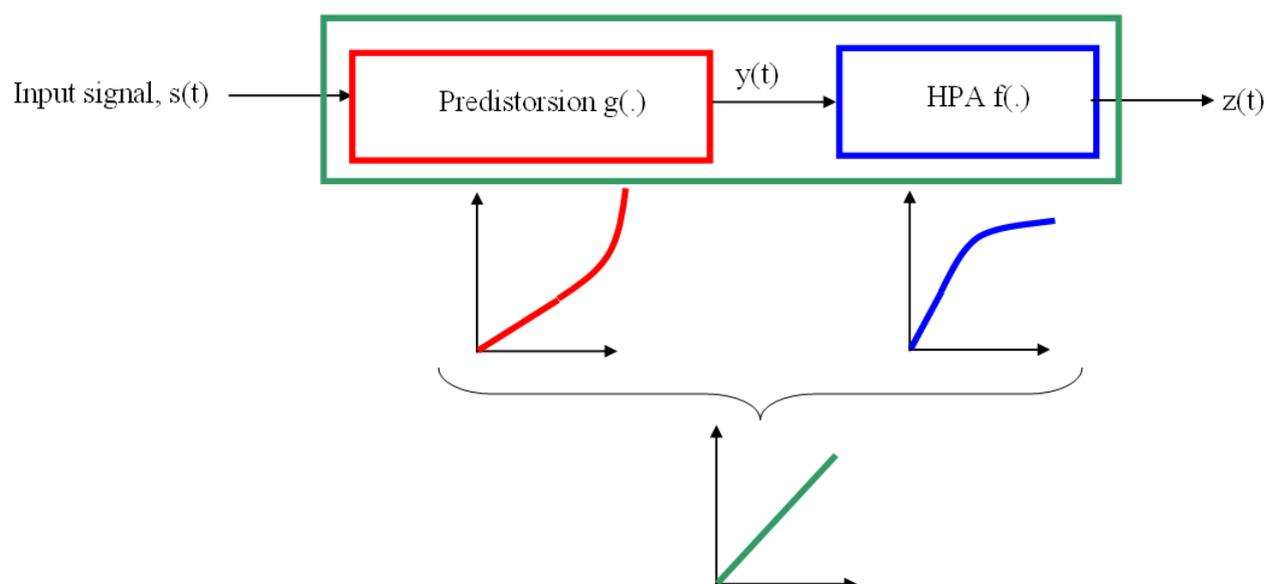
Figure 6-1: Principle of the predistorsion of a HPA.
