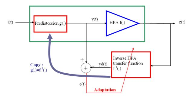
Figure 6-6: Indirect adaptation of the predistorsion function q(.).
