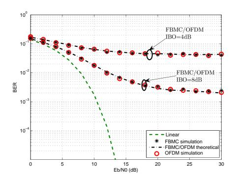
Figure 3-5: BER vs Eb/N0 for OFDM and FBMC system. Saleh HPA model, 64 subcarriers,  $16\text{QAM},\ \varphi_0=\pi/6$ , and AWGN channel.
