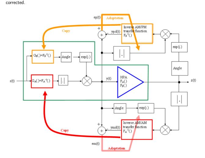
Figure 6-9: Modified NN-MLP architecture for FBMC predistorsion.
