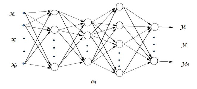
Figure 6-7: (a) Single Neuron, (b) Multi Layer Perceptron.
