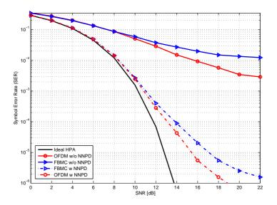
Figure 6-10: Performance of the first architecture based one a single NN-MLP.
