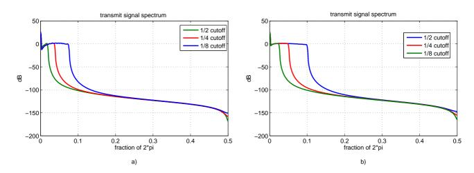
Figure 6-18: Transmit signal spectrum cutoff for uniform configuration (a), and non-uniform configuration (b) with oversampling factor 5:1.
