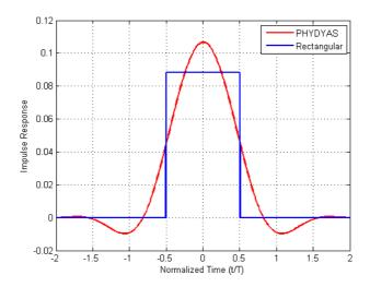
Figure 5-1: Impulse response for PHYDYAS and rectangular filters.
