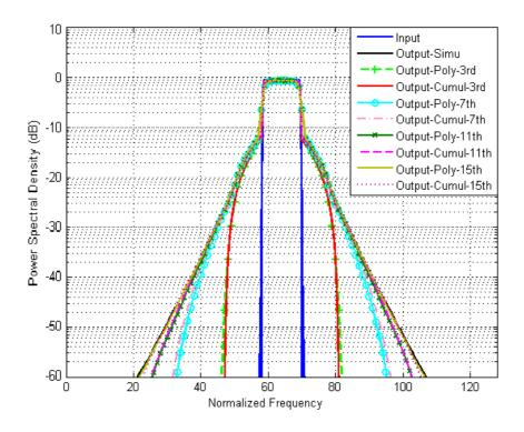
Figure 4-4: PSD Prediction with IBO=1dB.
