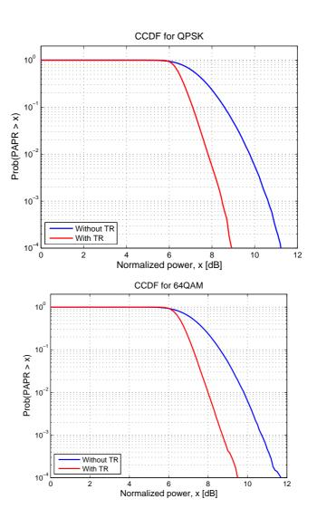
Figure 5-14: PAPR distribution with and without tone reservation in a FBMC case with 1.4 MHz LTE-like parameters for QPSK and 64QAM modulations.
