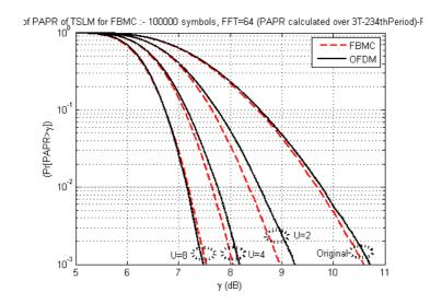
Figure 5-9: CCDF of PAPR plot for  $10^5$  FBMC symbols with PAPR calculated over [T,4T) with U=2,4,8 to illustrate the impact of size of U on the TSLM scheme in comparison with SLM scheme for OFDM.
