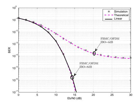
Figure 3-3: BER vs  ${\bf \it Eb/N0}$  for OFDM and FBMC system. SEL,  $A_{sat}=1$ , 64 subcarriers, 16QAM, and AWGN channel.
