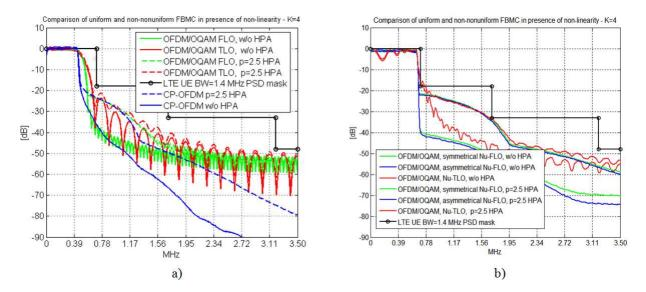
Figure 4-10: (a) Comparison of conventional OFDM, uniform FLO FBMC and uniform TLO FBMC, and (b) comparison of symmetrical Nu-FLO FBMC, asymmetrical Nu-FLO FBMC and Nu-TLO FBMC in context of HPA and mask fitting.
