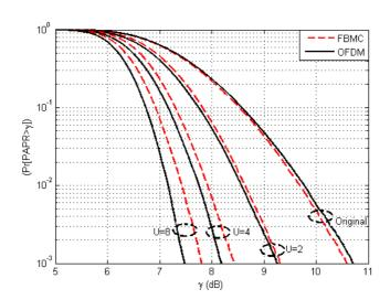
Figure 5-5: CCDF of PAPR plot for  $10^5$  FBMC symbols with PAPR calculated over [0,4T] with  $U=\{2,4,8\}$  to illustrate the impact of size of U on the DSLM scheme in comparison with SLM scheme for OFDM.
