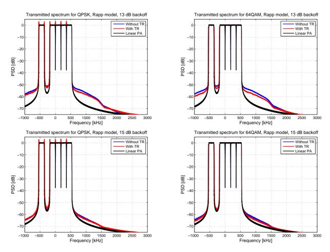
Figure 6-14: Spectral regrowth with 1.4 MHz LTE-like FBMC waveform with QPSK and 64QAM modulations and different back-off values using Rapp HPA model (p=2.25) with or without TR based PAPR mitigation.
