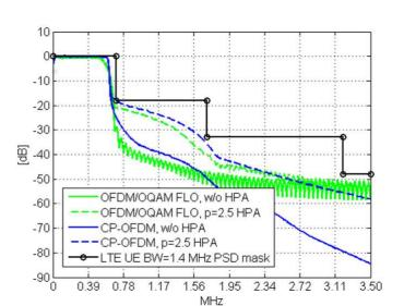
Figure 4-11: Comparison of conventional OFDM and uniform FLO FBMC for the maximum fitting of the PSD mask.
