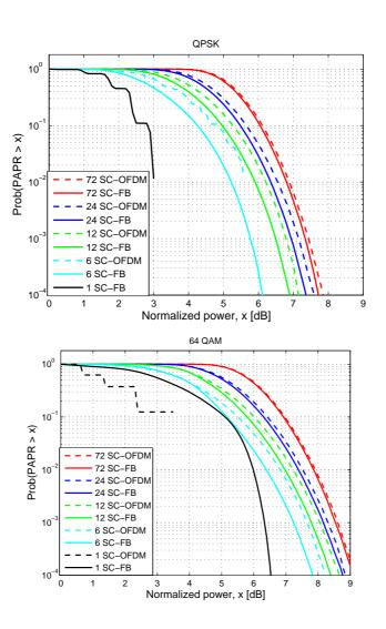
Figure 5-13: PAPR characteristics of OFDM based and FB based SC-waveforms with different bandwidths and roll-off factors. Upper: QPSK modulation. Lower: 64QAM modulation.
