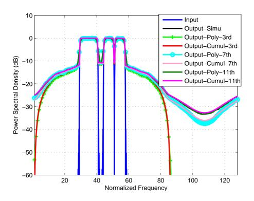
Figure 4-6: PSD Prediction with IBO=1dB (3 different active Sub-bands).
