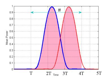
Figure 5-8: Power Profile of two FBMC symbols in the duration of  $\left[T,4T\right]$  w.r.t the current symbol.
