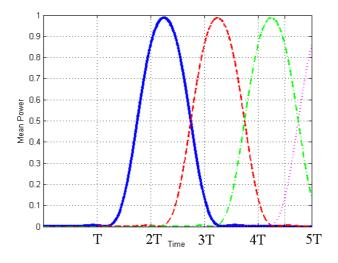
Figure 5-2: Illustration of mean-power overlapping among FBMC symbols.
