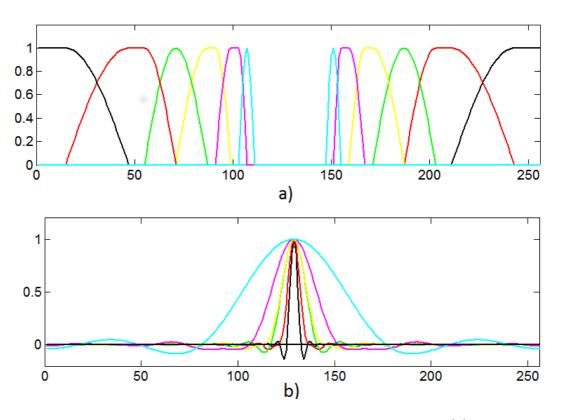
Figure 4-8: FLO Nu-FBMC arrangement with asymmetrical spectra (a) and corresponding time-domain representations (b) - all without oversampling.
