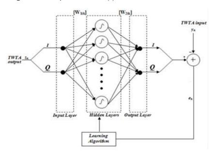
Figure 6-8: Multi Layer Perceptron for predistorsion.
