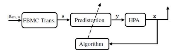
Figure 6-4: Principle of a baseband predistorsion.
