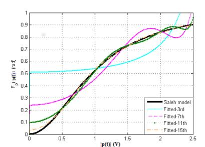
Figure 4-3: AM/PM distortion - Saleh Model and its polynomial fitting of orders 3, 7 , 11 and 15.
