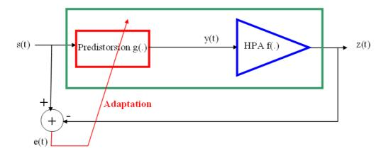
Figure 6-5: Direct adaptation of the predistorsion function g(.).
