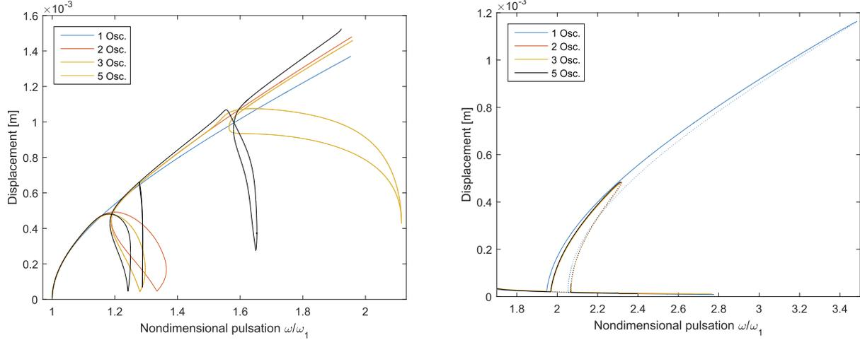
**Fig. 13.** Nonlinear free (left) and parametric (right) responses of the realistic bimorph of Fig. 12, computed with Manlab, with increasing number of bending modes in the ROM. All computations are performed with 10 harmonics in the HBM and the maximum transverse displacement over one period, at the center of the beam, is shown.
