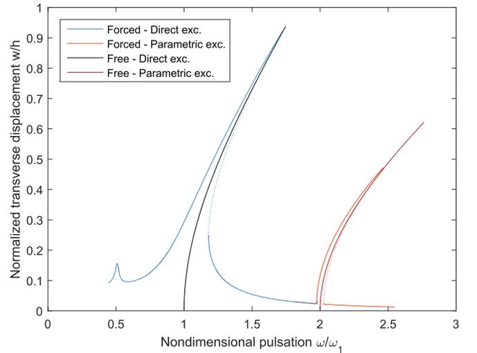
**Fig. 4.** Nonlinear free and forced responses of the hinged-hinged beam to the voltage signal  $V = V_0 \sin(\Omega t)$  with  $V_0 = 150$  V applied on the upper patch, computed with Manlab, with one mode in the ROM and 10 harmonics in the HBM. The maximum transverse displacement  $w$  over a period, at the center of the beam, normalized by the beam thickness  $h = h_b + 2h_p$ , is shown.
