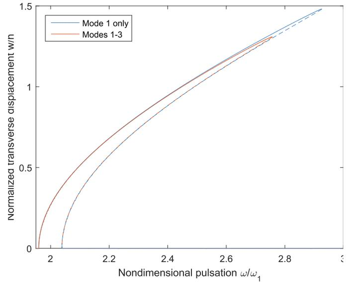
**Fig. 10.** Frequency response of the clamped–clamped beam of Fig. 5 at its first resonance with parametric excitation, computed with Matlab, with the first mode only and with the first and third modes in the ROM and 10 harmonics in the HBM. The maximum transverse displacement  $w$  over a period, at the center of the beam, normalized by the beam thickness  $h = h_b + 2h_p$ , is shown.
