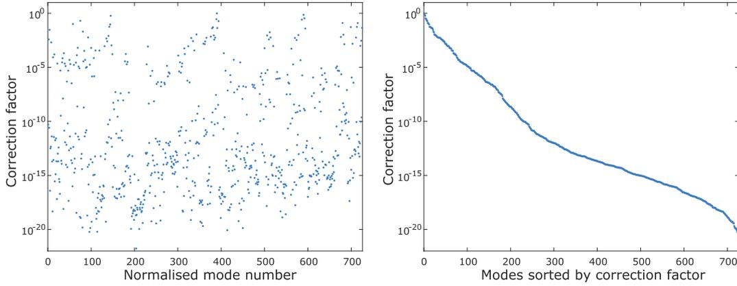
**Fig. 8.** Nondimensional correction factor  $\mathcal{F}_{11}^{s(\text{up})}/\Lambda_{11}^1$  of all the NB modes for the clamped–clamped beam of Fig. 5, sorted with the NB mode number  $s$  (left) and by decreasing correction factor (right).
