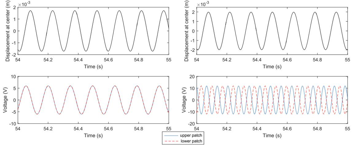
**Fig. 9.** Time signals of the displacements and outer electrode potentials, for the clamped–clamped beam of Fig. 5, in the steady state, computed with time integration in Abaqus, in the case of the direct (left) and parametric excitation (right).
