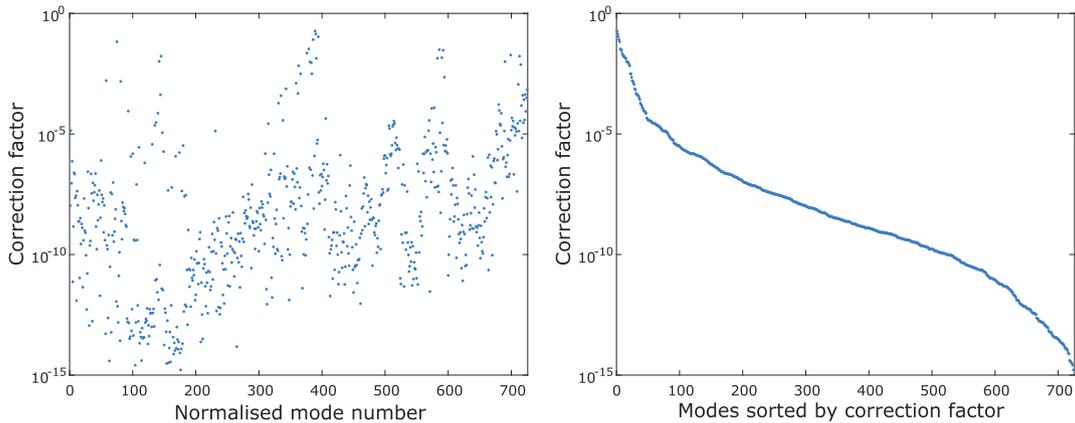
**Fig. 7.** Nondimensional correction factor  $\mathcal{G}_{111}^{1s}/\Gamma_{111}^1$  of all the NB modes for the clamped–clamped beam of Fig. 5, sorted with the NB mode number  $s$  (left) and by decreasing correction factor (right).
