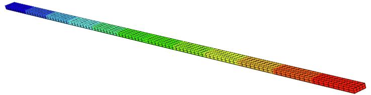
**Fig. C.15.** (a) Homogeneous, piezoelectric beam with load (traction applied on the second end) and boundary condition (clamped at the first end). (b) Result of the traction test on Abaqus with short-circuited electric BCs. The colors correspond to the displacements in the axial direction. (For interpretation of the references to colour in this figure legend, the reader is referred to the web version of this article.)
