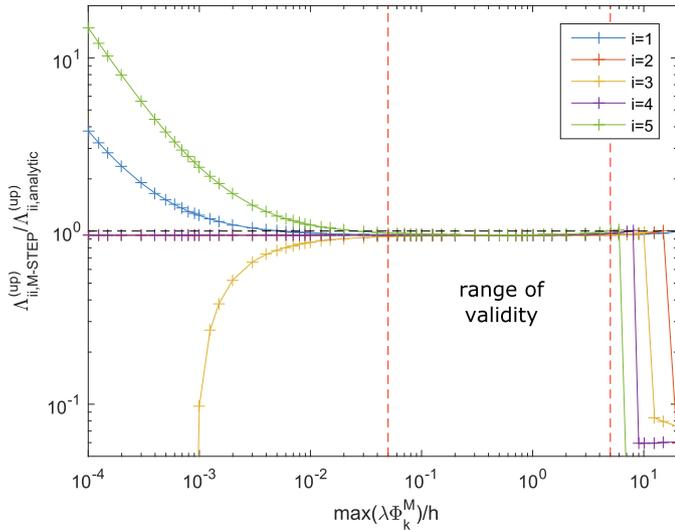
**Fig. 3.** Dependence of the parametric coefficient  $\Lambda_{ii}^{(up)}$  with regard to the prescribed displacement amplitude for different modes  $i = 1, 2, 3, 4, 5$ , computed by the M-STEP. Black dashed line: reference analytical value ( $\Lambda_{ii}^{(up),FE} = \Lambda_{ii}^{(up),AN}$ ). Red dashed lines: limits of the range of validity. (For interpretation of the references to colour in this figure legend, the reader is referred to the web version of this article.)
