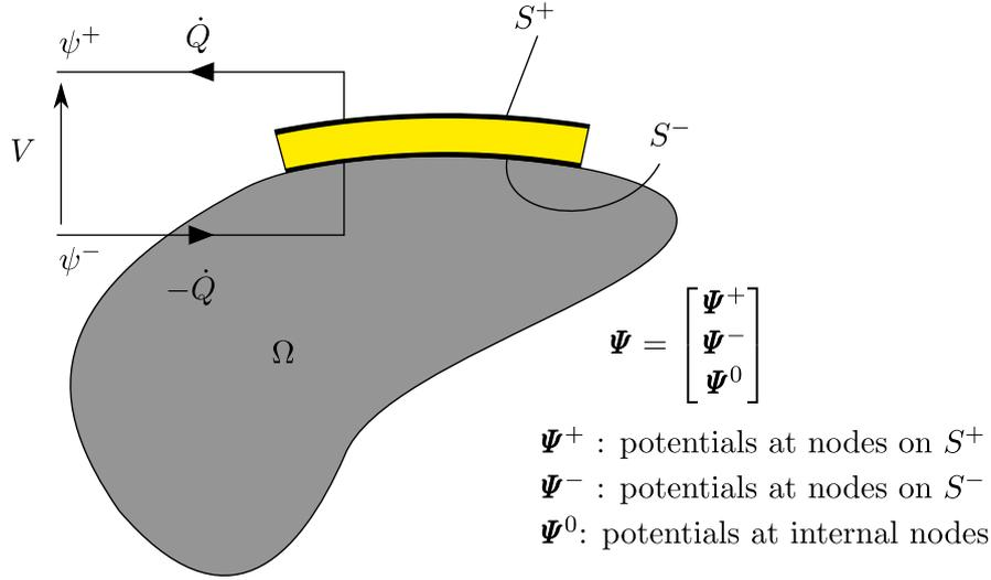
**Fig. 1.** Scheme of a whole piezoelectric structure with one patch. Elastic and piezoelectric materials are respectively represented in grey and yellow. (For interpretation of the references to colour in this figure legend, the reader is referred to the web version of this article.)
