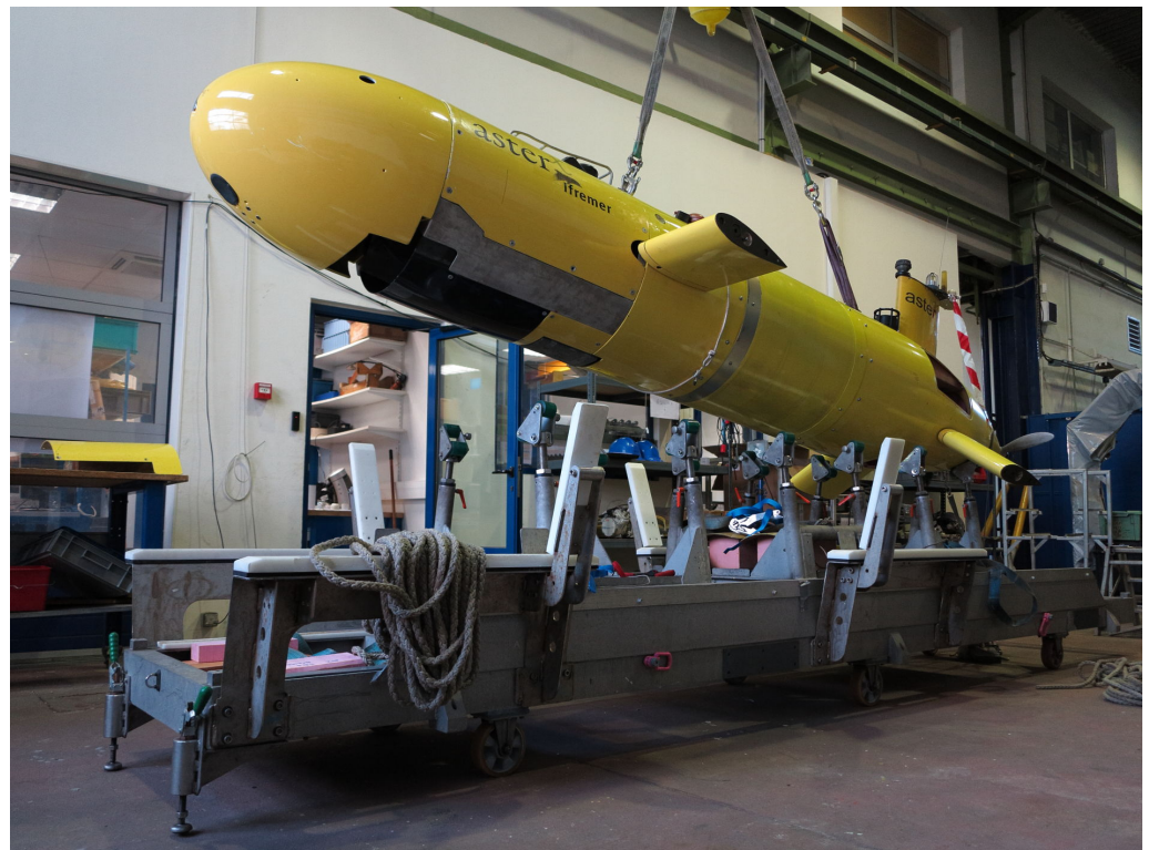
Figure 3. View of the AUV during the manipulation performed to adjust the internal parameters of the GraviMob system in one of the tilted positions. The AUV can thus be tilted along the roll, pitch and yaw axes.
