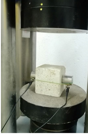
Fig. 3 Uniaxial compression apparatus with ultrasonic transducers.
