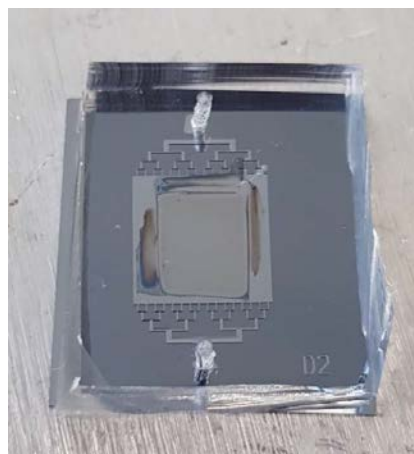
Figure 1: Photography of the microfluidic growth chip showing the wide growth chamber and the flow distribution trees.
