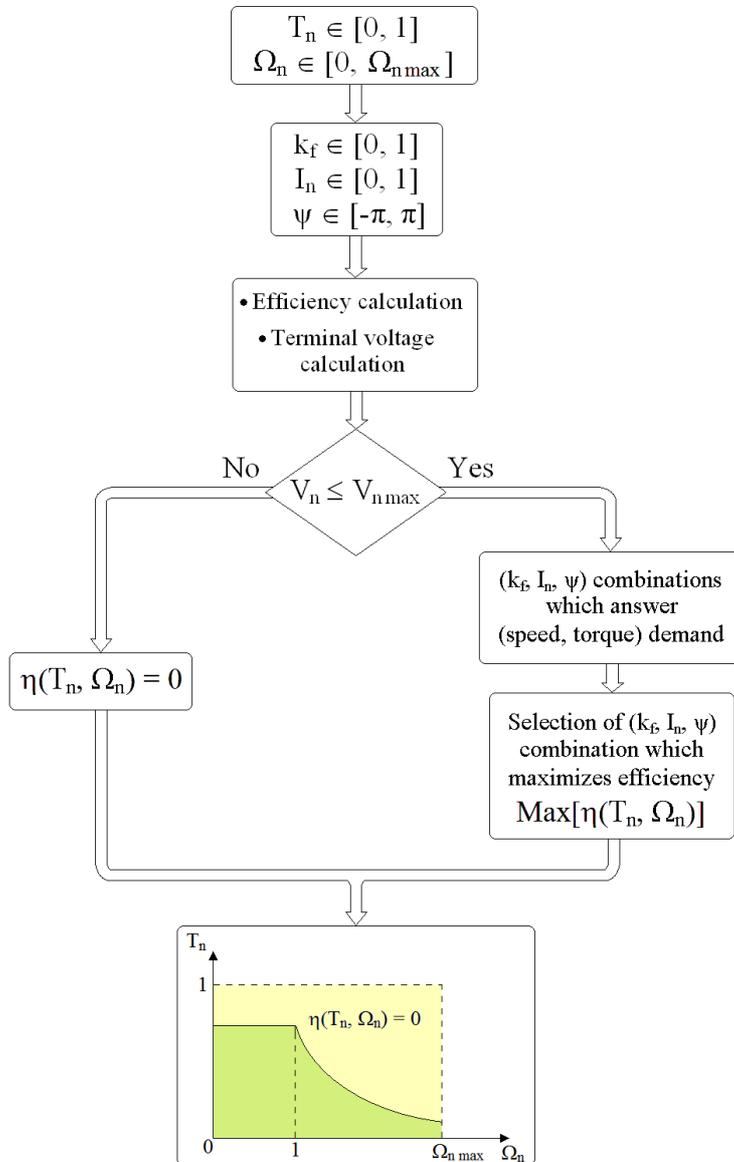
Fig. 6. Efficiency maps computation algorithm.
