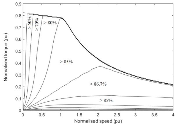
Fig. 8. Efficiency map of the HESM ( $\alpha = 0.5$ ).
