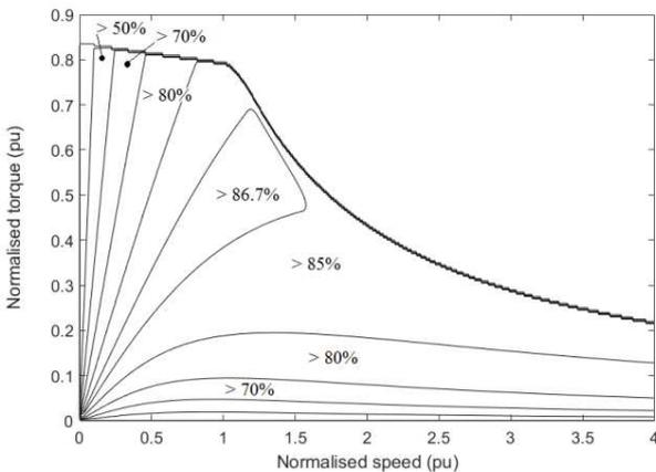
Fig. 7. Efficiency map of the HESM ( $\alpha = 1$ ).
