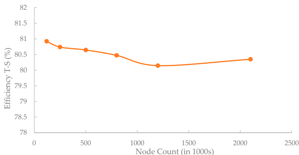
Figure 3. Mesh refinement study based on total-to-static efficiency evolution over number of nodes.
