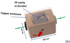
Figure 5: Project design of our new quantum pascal realization set-up. (a) 50 mm single Fabry-Perot (FP) resonator composed of two silica mirror and a spacer made in Zerodur<sup>®</sup>. (b). Cross section of the copper enclosure including the FP resonator.
