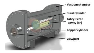
Figure 2: Cross-section of the vacuum chamber with a Fabry-Perot cavity. Fabry-Perot resonator composed of two silica mirrors and a spacer made in Zerodur<sup>®</sup>.
