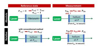
Figure 3: Schematic of the two methods (absolute and relative) to determine a pressure using a refractometer. P is a pressure, n is the refractive index et  $\nu$  the frequency. ref index indicates the reference state of the parameters and He index indicates the measurement state.
