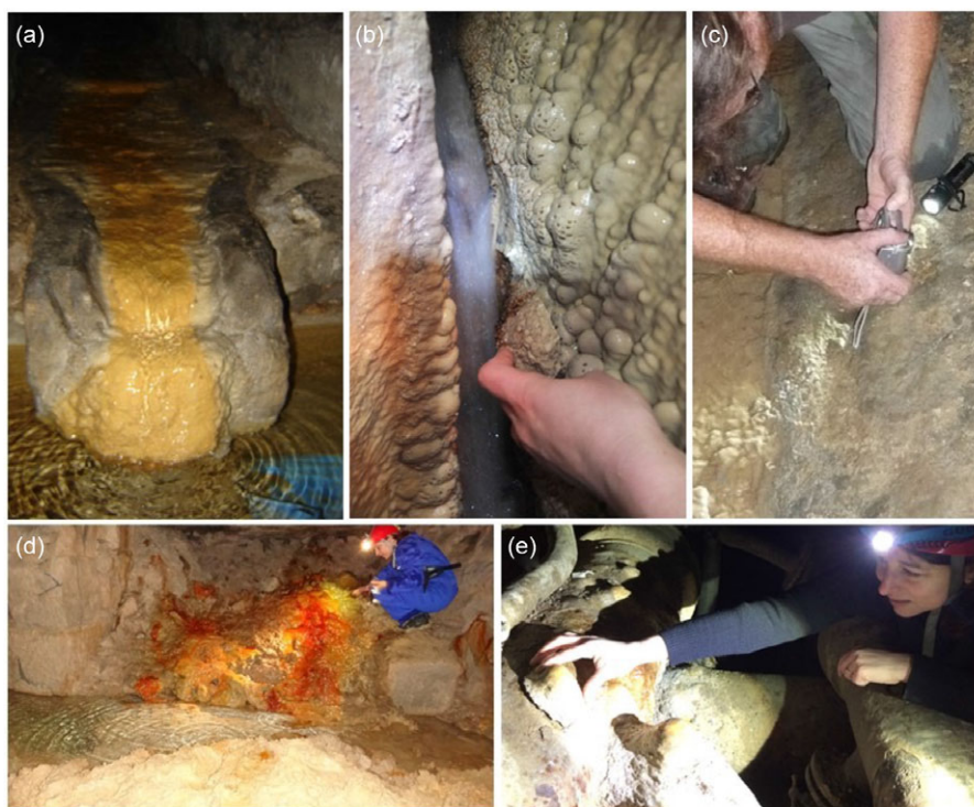
Figure 2 Pictures of the studied sites: (a) historical fountain of Saint Martin Manhole with \text{CaCO}_3 crust (sample SM B); (b) Rungis aqueduct, south of Paris, with sample Run1 at the time of its collection in a water inlet; (c) Belleville aqueduct in northern Paris, and Bra 1 sample at the time of its collection; (d) Brasserie former quarry, with the red carbonate crust sampled (Bra 1 sample); (e) under the Neptune basin, Versailles Palace Gardens, Nep 2 sample, deposited on a pipe, by the fountain and basin leakages. (Please see online version for color figures.)
