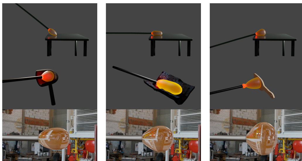
Figure 20. Computer-aided, VR presentation of glass making processes from [45]. Top: Marvering. Middle: Shaping. Bottom: Illustration of the glass deformation during glass blowing.
