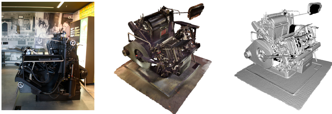
Figure 23. Digitisation of Machines for mastic processing.
