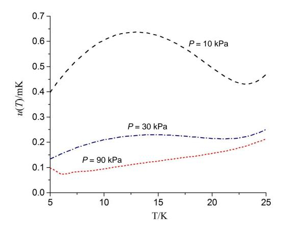
Figure 6. Total uncertainty expected in temperature measurements referred to the triple point of neon (24.6 K), for fixed gas pressures in the range 10 kPa to 90 kPa. Key: ----- P=10kPa;  $-\cdot---$  P=30kPa; ----- P=90kPa.
