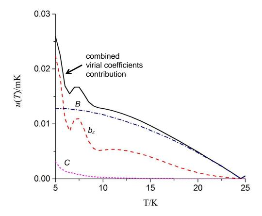
Figure 2. Expected contributions to the uncertainty due to the virial coefficients B, C, and  $b_{\varepsilon}$ , for temperature measurements referred to the triple point of neon (24.6 K). The hump near 7 K is due to values of uncertainties for B given in the literature [2]. Key: ---- dielectric virial coefficient  $b_{\varepsilon}$ : ------ virial coefficient B; — combined uncertainty due to virial coefficients.
