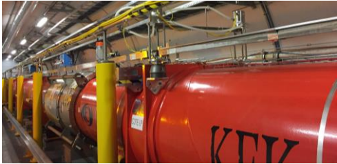
LHC / HL-LHC full remote alignment system for the Low-β quadrupoles
