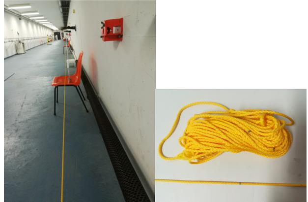
Figure 4: Left: the stretched wire along the longitudinal axis of our test laboratory. Right: the stretched wire, a 2 mm diameter polypropolen builders line, with marks done with a pen.
