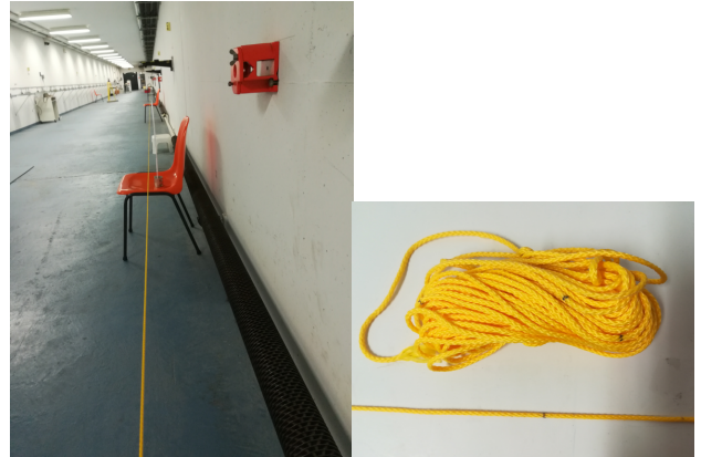
Figure 4: Left: the stretched wire along the longitudinal axis of our test laboratory. Right: the stretched wire, a 2 mm diameter polypropolen builders line, with marks done with a pen.
