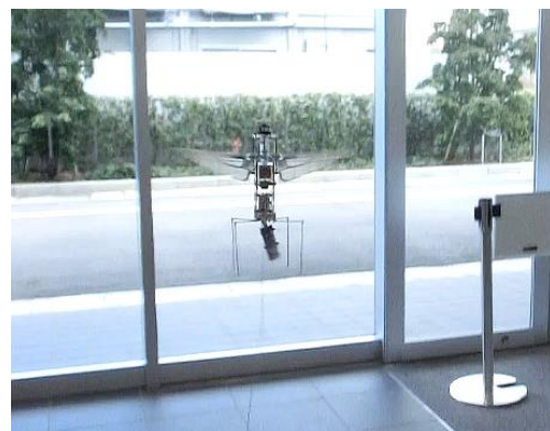
Figure 1: The developed tailless two-winged FMAV and the wireless autonomous flight.
