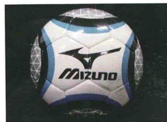
(b) Type A-ball, +Teamgeist, Molten. (c) Type B-ball, truncated icosahedron, Mizuno Figure 4-3 Time-averaged drag coefficients of a sphere with smooth surface and soccer balls at various Re numbers. Type A-ball, Type B-ball.
