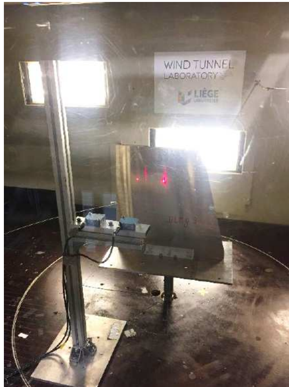
Figure 5: Cantilevered flat plate wing in wind tunnel
