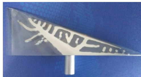
Figure 5: 3D print of topology optimization structure.
