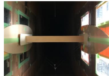
Figure 1: Section model for spring-supported tests mounted in Kyushu Institute Technology wind tunnel
