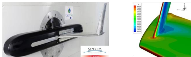
Figure 1: Flutter model wall-mounted in the test section of the transonic pressurized wind tunnel S2MA (Onera) (2016) – Pressure distribution at the empennage intersecting surfaces.
