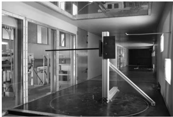
Figure 11: 4:1 rectangular cylinder in wind tunnel
