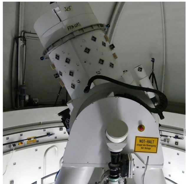
Fig. 7 Local reference frame with certificated scale-bars and photogrammetric targets as well as the prepared Satellite Observing System Wettzell
