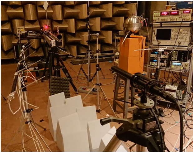
Fig. 2 Simultaneous measurement of the speed of sound by differential distance change (foreground) and by the cavity resonance method in an anechoic chamber (sphere in the background) for verification and reduction of uncertainty of the Cramer equations
