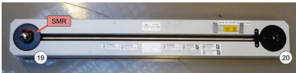
Figure 13. Photograph of the Leica scale bar, with on the left a SMR installed on the nest.
