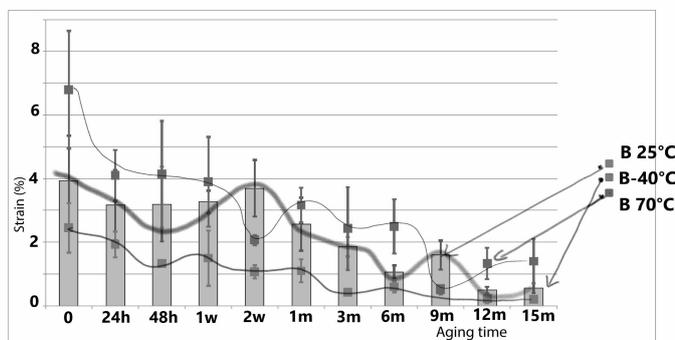
Fig. 5. Evolution of the deformation of system B as a function of the aging time and the test temperature.
