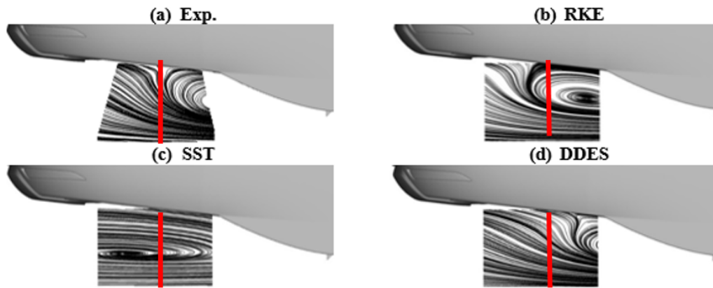
Fig. 23: Comparisons of streamlines in the wake of the rear right fairing between experiments and computations.
