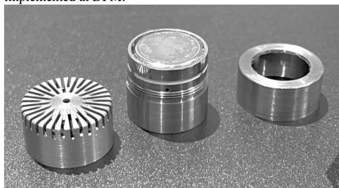
Figure 8 The Brüel and Kjær type 4134 microphone with its regular protection grid (left), and UA0825 adapter (right) for converting to laboratory standard configuration. The microphone pressure-equalisation vent outlet is visible just above the thread.
