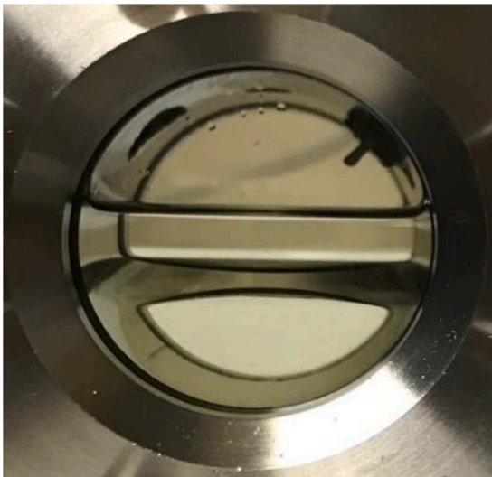
Fig. 3. Refrigerant not fully miscible in oil, immediately after refrigerant filling.
