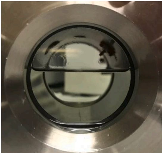
Fig. 4. Example of Propylene miscible in PAG oil.
