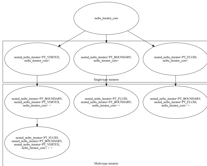
Fig. 8. Chain inheritance through nesting class templates. Single-type iterators derive directly from the core class, multi-type iterators derive from the other multi- or single-type iterators. For multi-type iterators, the order of the nesting determines the order in which neighbor types are processed. On the middle, for example, fluid types are processed before boundary types, whereas on the right boundary types are processed first.
