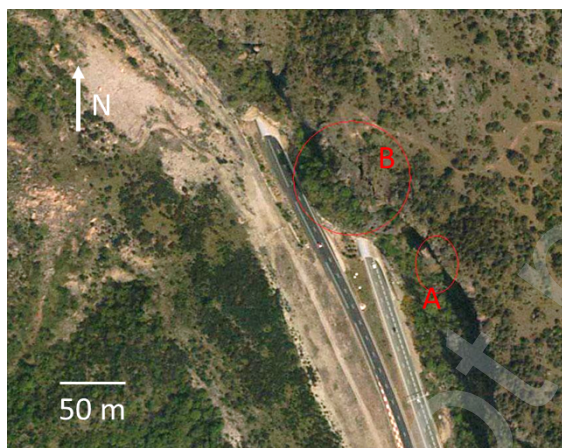
90 Figure 1: Location of the site and geological clues. a- general view of the columns and 91 simplified geological interpretation b-Top view of the site - red circles show the large 92 fractures that separate the columns from the cliff; c- Geological map of the area, the highway 93 is in red, the tunnel is in dotted line. 94
