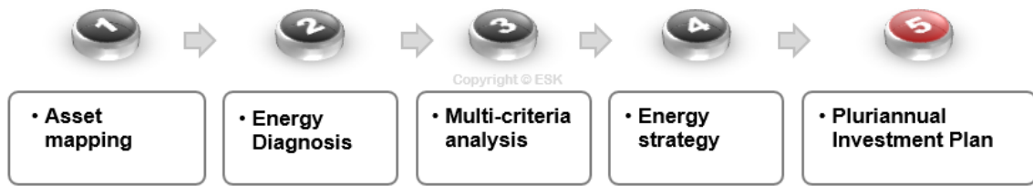
Activities ranging from 3 to 18 months to identify a Certification Scope (CS) dedicated to the ISO 50001 standard, depending on the number of assets in a community.
