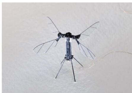
**Figure 9.** Miniature robot with insect-like flight capabilities, [119].
