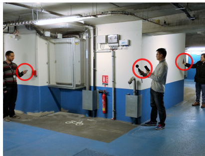
(b) Underground calibration : Three persons speak in a quiet parking. All are holding their devices next to a wall, while the person in the middle additionally holds a SLM that serves as ground truth.
